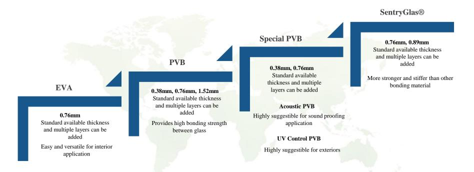
Laminated glass is basically a glass sandwich. It is made of two or more plies of glass with a vinyl interlayer (EVA /PVB /SGP) between.
